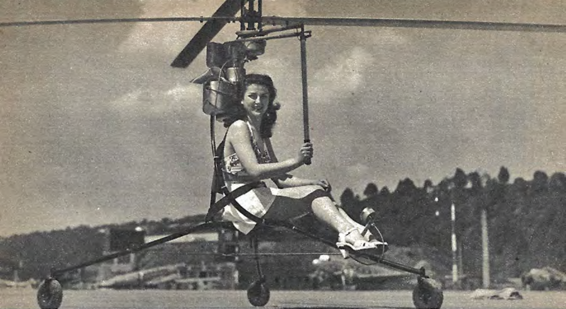
Second version of the Hoppicopter design had a tripod landing gear with motor mounted behind the pilot's head. It was better than the original "back strap" model but weight distribution was unsatisfactory.
