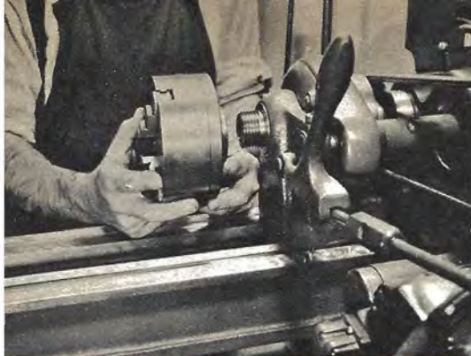
Ends of the brass rod for the upright will have to be squared off and drilled for center holes. The rod will be gripped in this three-jaw chuck.
