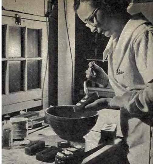
Small quantities are made completely by hand but for larger orders molds are prepared into which the liquefied materials are then carefully poured.
