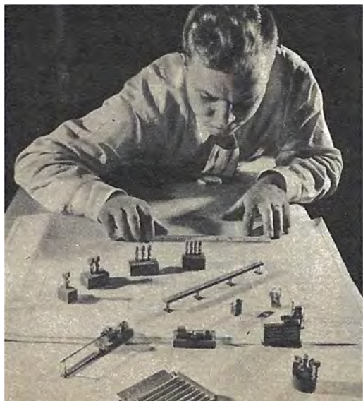
Tool drawing specifications are checked against models of various machine tools. Note the tiny conveyors, rolling mills and multiple drill presses.
