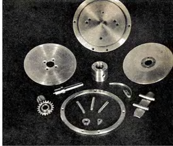
Left: The 5-in. diameter jig fixture to which all the disks are screwed while machining. Right: Parts ready for assembly.
