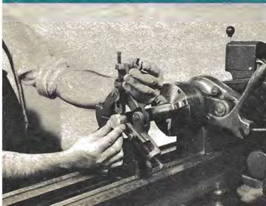
End of rod is retained by this steady rest, which has individually adjusted jaws. After jaws are positioned by end screws, tighten bolts as shown.
