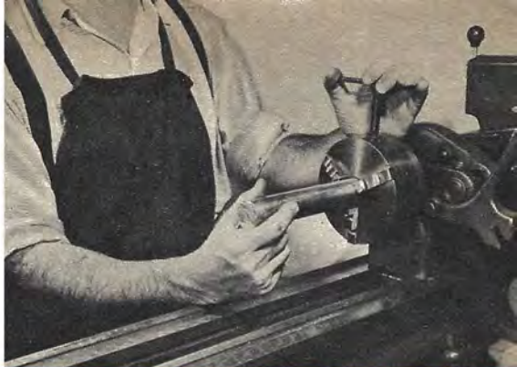
Supporting free end of candle holder rod, tighten chuck. Jaws are self-centering so that they all move simultaneously when key is turned.
