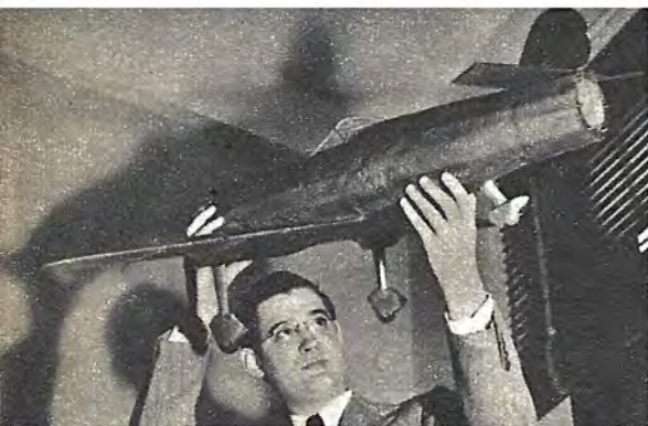
Mother bomb, top, holds five smaller bombs which scatter in all directions on impact. Rocket propeller ship, above, has a hollow hull to insure greater speed by cutting down wind resistance.
