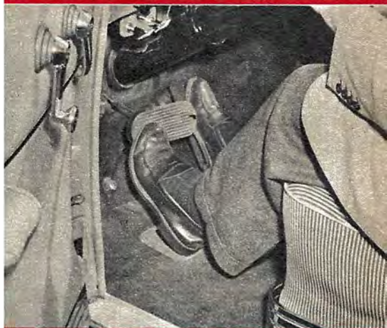
On cars equipped with automatic transmission Studebaker has widened the brake pedal, thus letting the driver operate it with either foot.
