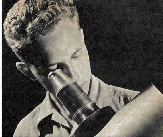
Close-up of the eyepiece construction. The ocular he is using is one designed for richest-field observation. The adapter was turned on a lathe.
