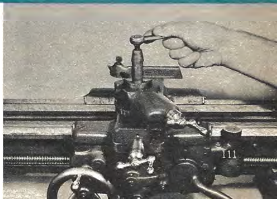
Since tool holder takes force of revolving work it must be well tightened. Side-facing bit is in holder preparatory to facing end of the rod.
